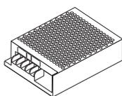
ALIMENTATORE switching 12Vdc - 42W
